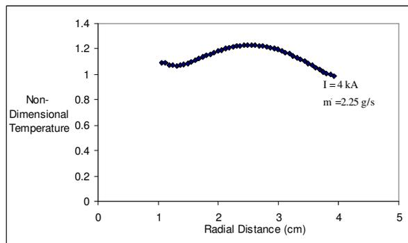
Figure17: Exit temperature distribution versus radial distance
