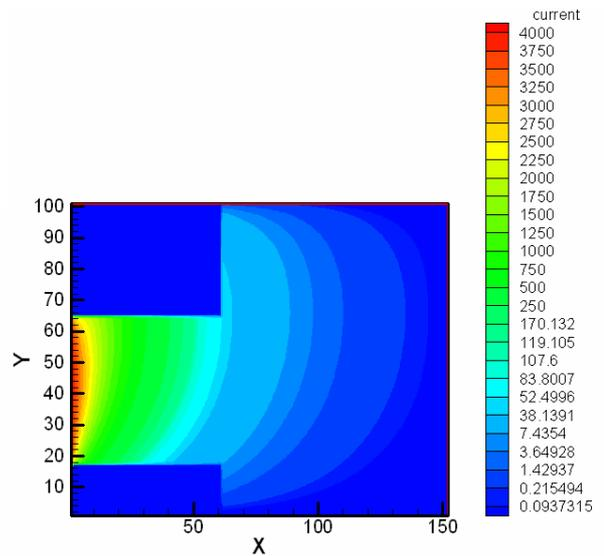
Figure10: Contours of electrical current for  $I_\infty = 4kA$
