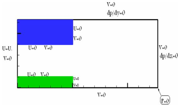
Figure3: The velocity boundary conditions for MPD thruster
