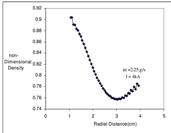
Figure16: Exit density distribution against radial distance
