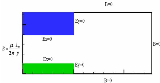
Figure5: The electromagnetic boundary conditions for MPD thruster
