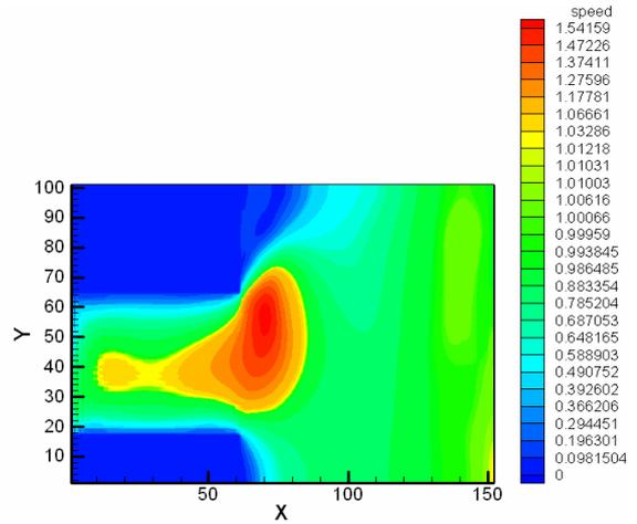
Figure9: Velocity contours for  $I_\infty = 4kA$
