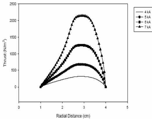
Figure14: Exit thrust vs. current [7]
