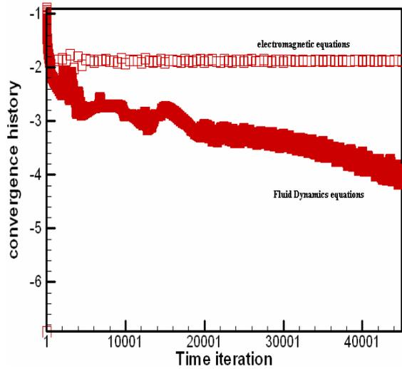
Figure18: Residual of density against time iterations ( $I_{\infty} = 4kA$  and  $\dot{m} = 2.25 \frac{g}{s}$ )
