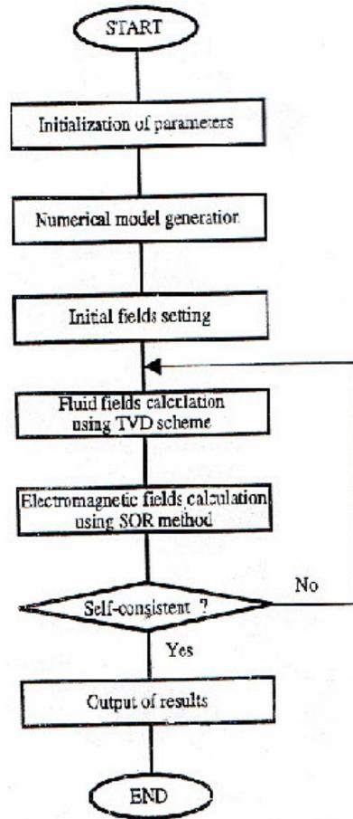
Figure2: The flowchart of numerical algorithm for analyzing MPD thrusters
