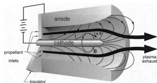
Figure 1: A schematic of a magneto plasma dynamic thruster (MPDT)
