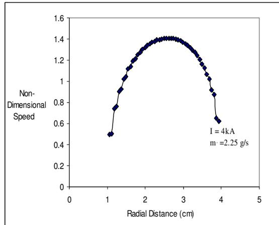
Figure15: The exit velocity versus radial distance
