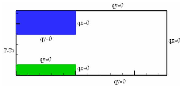
Figure4: The thermal boundary conditions for MPD thruster
