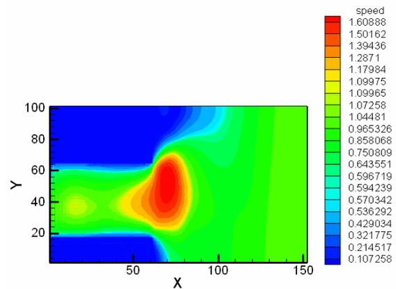
Figure11: Contours of velocity for  $I_\infty = 5kA$
