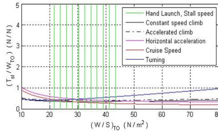
**Fig .2.** Constraint analyses for the IUT MAV2013
