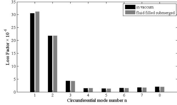
**Figure 4.** Comparison of coupled and uncoupled loss factors ( $m = 1$ ), although both real and imaginary parts of natural frequency has changed the loss factor has slight changes because fluid has been assumed inviscid.
