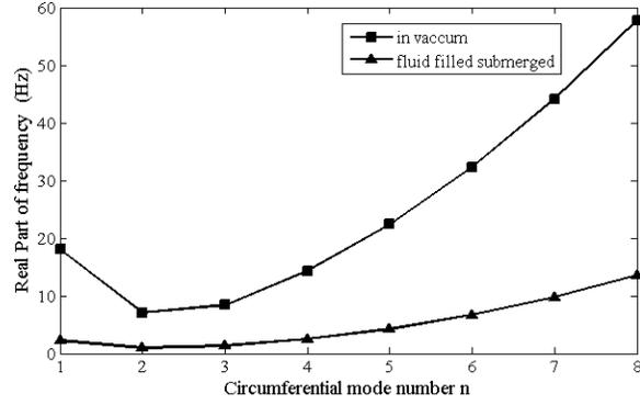
**Figure 2.** Comparison of coupled and uncoupled real part of frequency ( $m = 1$ ) for a viscoelastic shell, because of fluid added mass the variation of real part remains similar to that is discussed in [10] for a elastic shell.
