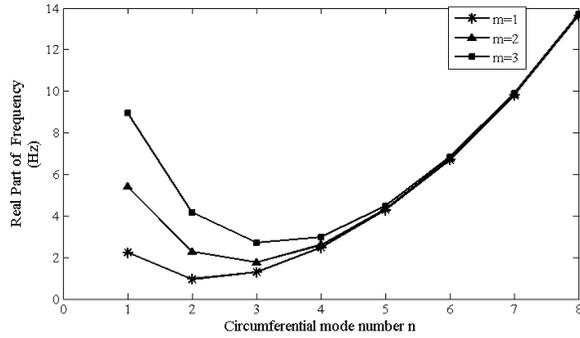
**Figure 5.** Variation of real part of natural frequency in different axial wave numbers when  $n$  is increasing for a fluid filled submerged cylindrical shell  $L = 20$  m,  $R = 1$  m,  $h = 1$  cm, this variation is similar to that of an elastic shell.
