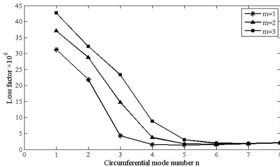
**Figure 7.** Variation of loss factor of natural frequency in different axial wave numbers when  $n$  is increasing for a fluid filled submerged cylindrical shell  $L = 20$  m,  $R = 1$  m,  $h = 1$  cm , although for high  $n$  the real part is increasing and imaginary part is almost unchanged, the loss factor is unchanged.
