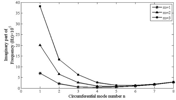
**Figure 6.** Variation of imaginary part of natural frequency in different axial wave numbers when  $n$  is increasing for a fluid filled submerged cylindrical shell  $L = 20$  m,  $R = 1$  m,  $h = 1$  cm, this variations follow an unpredictable trend which is different from real part, and when  $n$  is high imaginary part remains almost unchanged.
