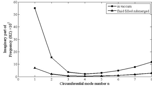
**Figure 3.** Comparison of coupled and uncoupled imaginary part of frequency ( $m = 1$ ) for a viscoelastic shell, fluid has a similar effect on imaginary part and variation is similar to that of real part.
